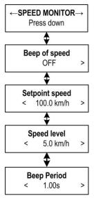
*Beep of speed* – Set the independent audible speed indicator. This does not affect the alarm.
