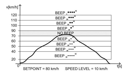
**CONTROL SIGNAL** – By pressing the Down key, we can modify options relating to the input control signal. This allows simple switching on/off of the audible alarms generated by MSPEED.
