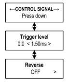
Trigger level – Set the trigger speed for recording of data. For example if the trigger level is 1.50ms and Reverse is OFF, as soon as a speed of 1.50ms is exceeded, then data recording begins and any previously recorded maximum/minimum values are deleted. If the speed is less than the trigger level, no data is recorded and previously recorded data remains unaffected. No acoustic signalling will be given in this case.
