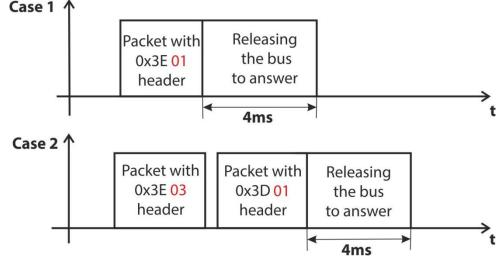
The figure above is a schematic diagram of both cases of the packet generated by the Master.
